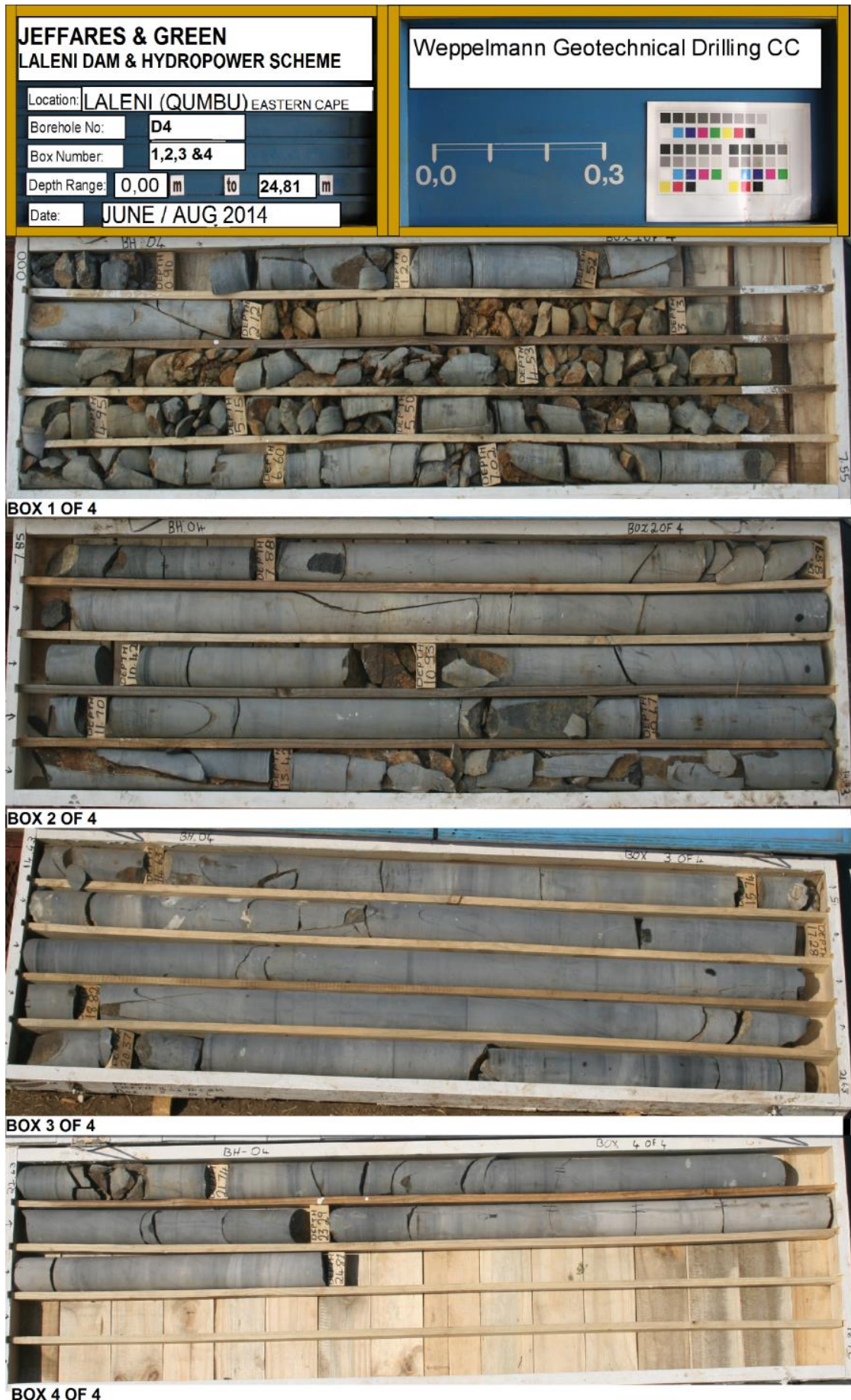
Fig B-8: Borehole D4 – Box 1 to 4 Dry
