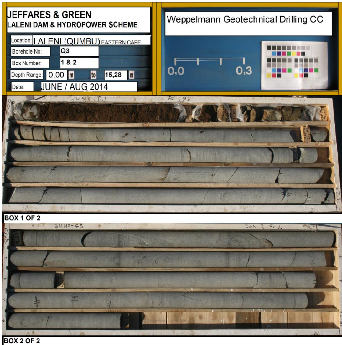
Fig C-6: Borehole Quarry 3 – Box 1 to 2 Dry
